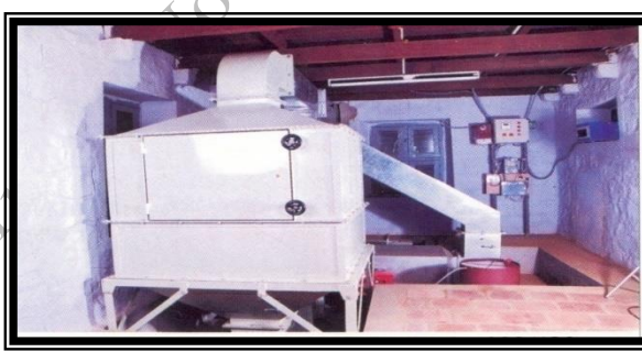
Fig. 5.37: Modern cardamom curing chamber
